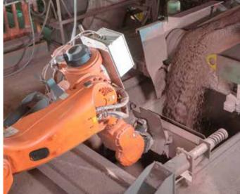
Sinter raw mix sampling during conveyor discharge
