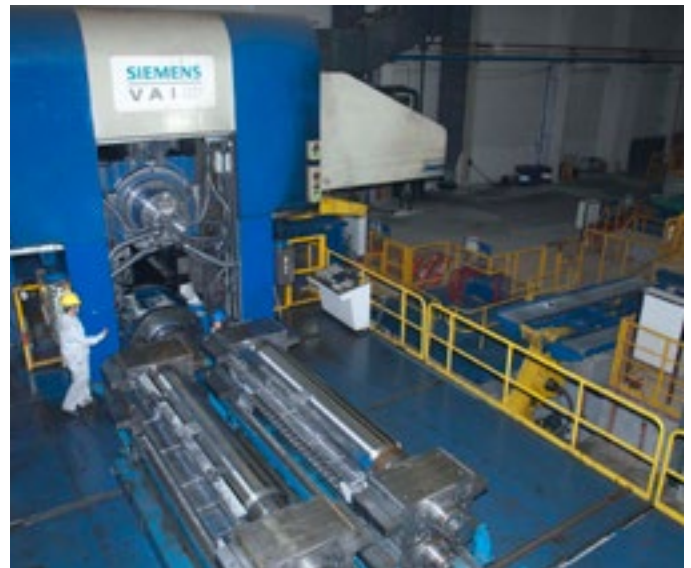
Completion of the work roll change at Henan
